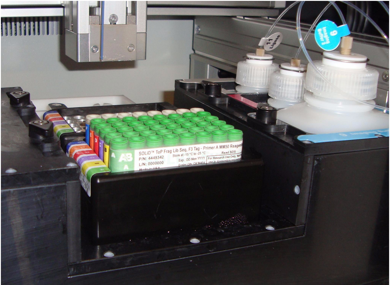
Figure 28 Position of the sequencing reagent blocks for flowcells 1 and 2.
