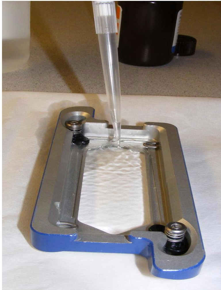
Figure 8 Cover the slide completely with SOLiD™ XD Slide Prep Reagent and let sit for 2 minutes—do not let it dry out.
