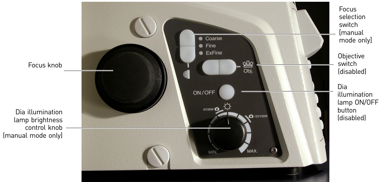
Figure 13 Nikon Eclipse Ti-E left operation panel
