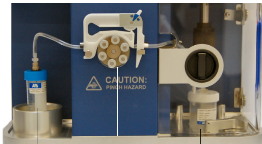
Figure 3 Emulsifier interior components
