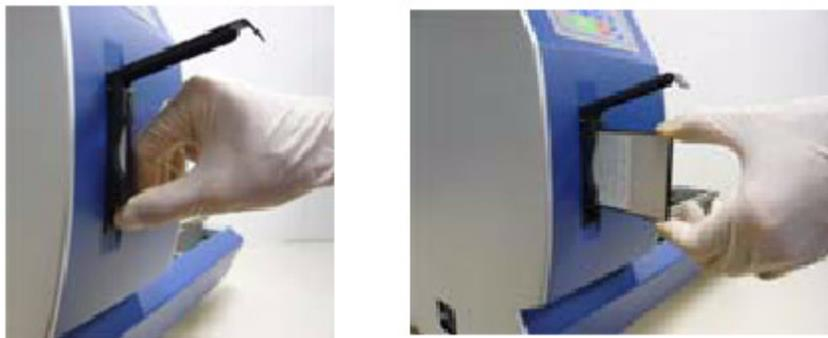
4. Insert the appropriate protocol card in the slot with the arrow on the protocol card pointing toward the instrument and the label facing left.
