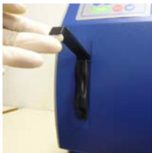
3. To remove a card that is already installed in the slot, push the button located below the card slot (see the photo below), then pull the card out of the slot. Place the card in the plastic cover in the box.
