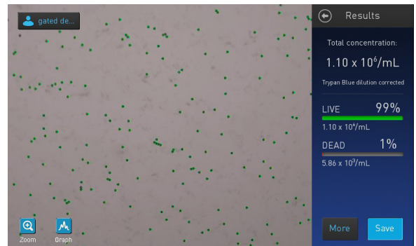
After gating – accurate results when debris is excluded from cell count
