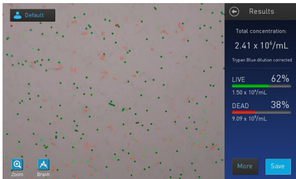
Before gating – debris counted as dead cells result in falsely high dead cell count
