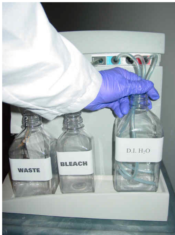
Figure 7.5 Immerse the three wash and water lines in the DI water bottle.
