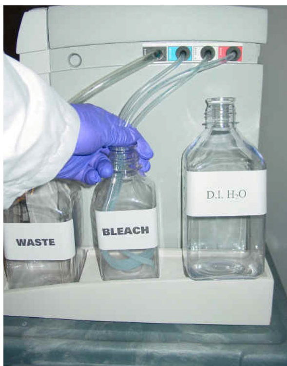
Figure 7.2 The bleach cycle. Immerse the tubes into the 0.525% sodium hypochlorite solution. The waste line remains in the waste bottle.
