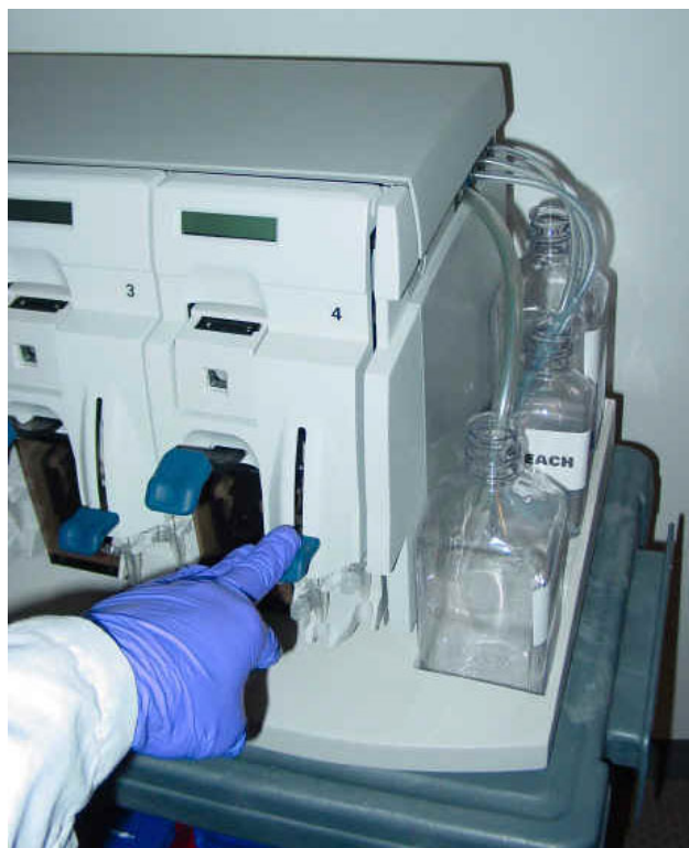
Figure 35 Press down on the needle levers to start the bleach protocol.
