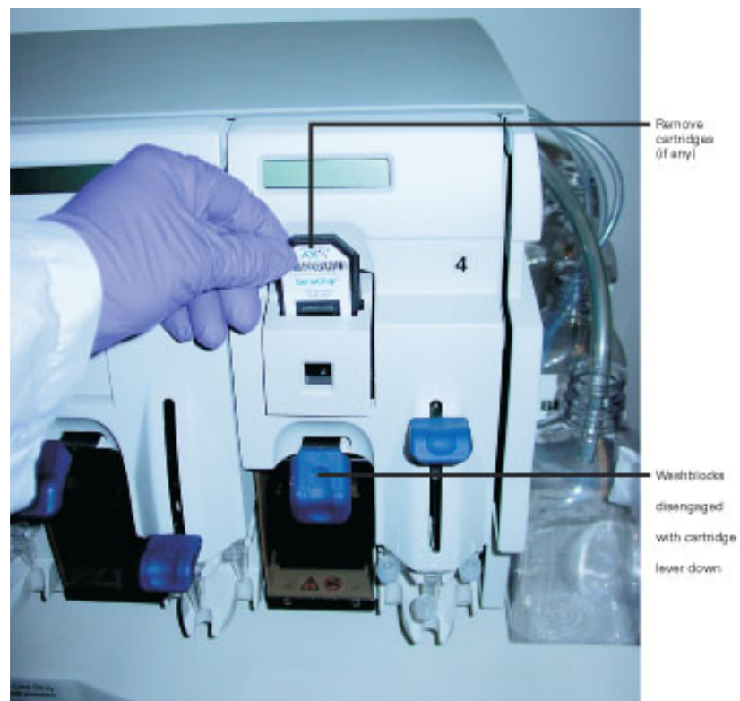
Figure 32 Disengaged washblocks showing cartridge levers in the down position. Remove any cartridges.
