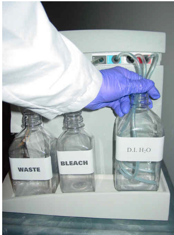
Figure 36 Immerse the three wash and water lines in the DI water bottle.
