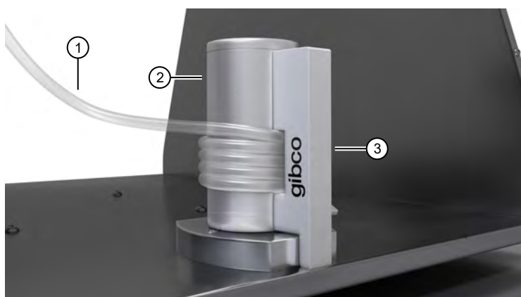
Figure 4 Tubing wrapped four times around the Secondary Magnet
