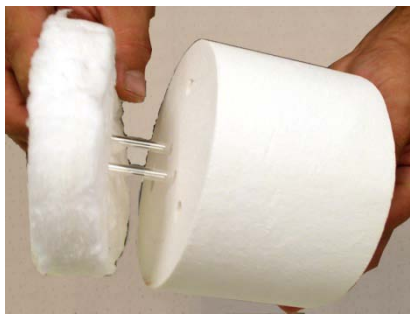
Figure 10–17. Application de l'isolation Kaowool
