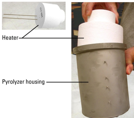
Figure 10-7. Insert replacement heater into housing
