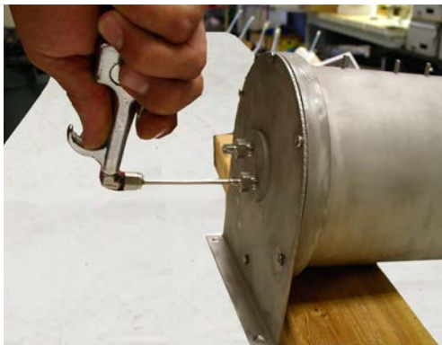
Figure 10–14. Blow out the debris
