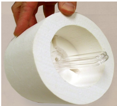
Figure 10-16. Pyrolyzer tube inserted into the insulation
