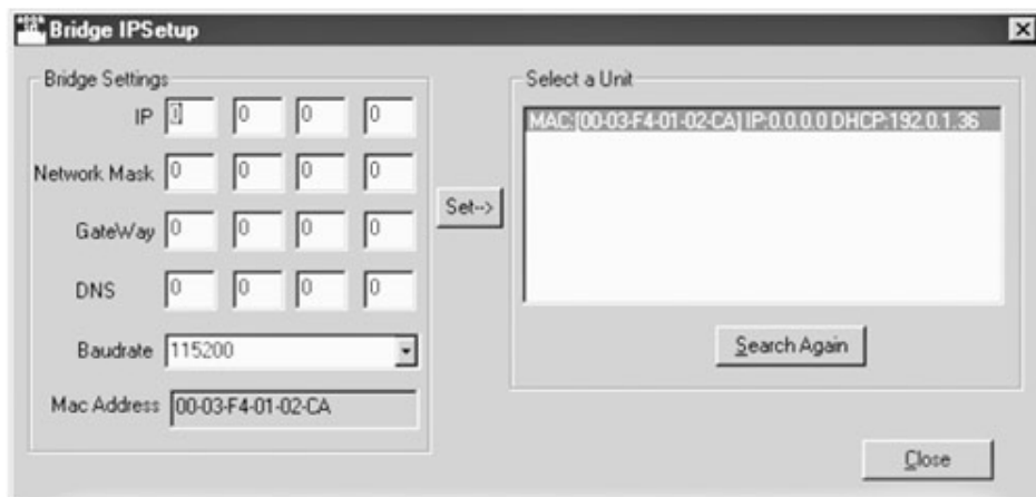
Figure D-3. Example display with DHCP server present
