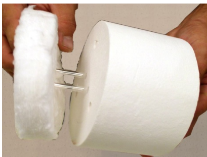
Figure 10-17. Apply the Kaowool insulation
