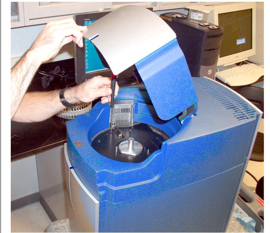
5. Use a standard, flat (-) screwdriver and gently slide it down through the hole making sure not to damage the shaft and spring that are protruding into the hole. When the screwdriver stops, it should be in contact with the Scanner Y stage screw. Slowly turn the screwdriver until you feel it engaging the slot on the screw of the scanner Y stage.
