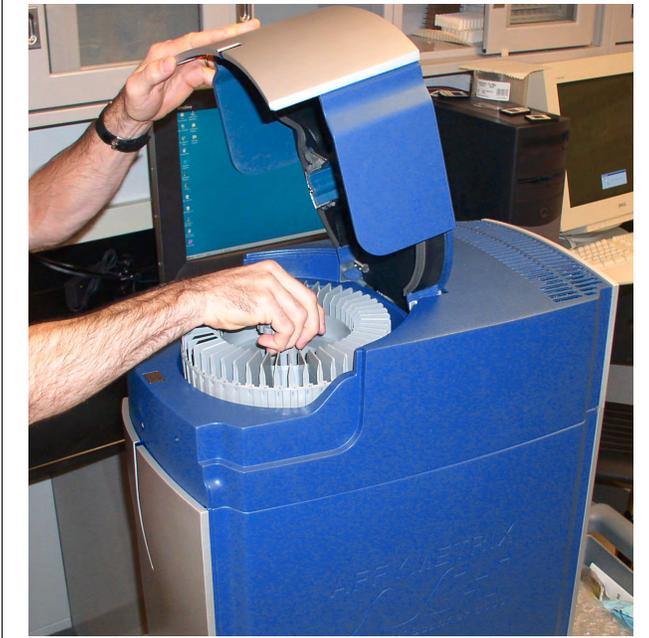
**NOTE:** You may have to turn the carousel several times before it seats into the alignment pin and alignment key. When seated properly, the carousel is flush with the AutoLoaderDx v.2 housing. The seating of the key flat is confirmed by a gentle falling of the carousel into the key.
