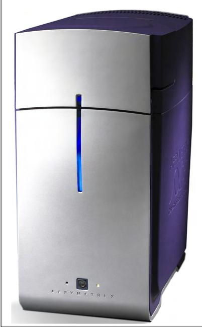
The Scanner 3000Dx v.2 with AutoLoaderDx v.2 (Figure 2.3) is a wide-field, epifluorescent, confocal, scanning laser microscope. It scans the chip after staining on the Fluidics Station 450Dx v.2. Array cartridges are loaded into the scanner by the AutoLoaderDx v.2 (an automatic handler) before scanning and returned to the AutoLoaderDx v.2 when scanning finishes.
