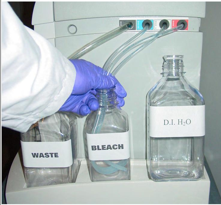
6. Immerse all three wash and water lines of the fluidics station into the 500-mL bottle of bleach solution (Figure 4.17). Do not immerse waste line into bleach.
