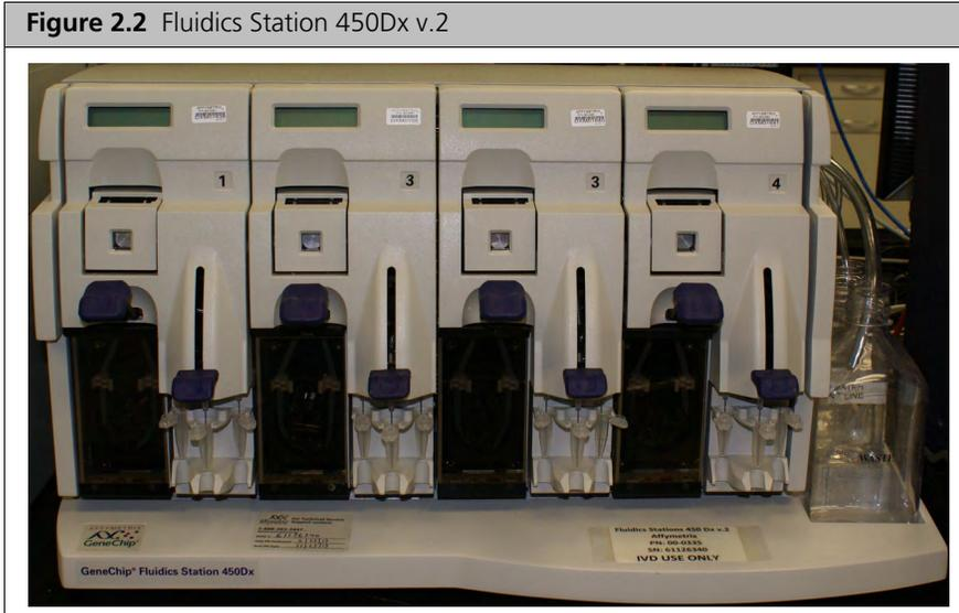
The Fluidics Station 450Dx v.2 (Figure 2.2) consists of four modules installed in a single housing. Each module holds a single array and performs the hybridization, washing, and staining functions for that array. Up to eight stations can communicate with one system workstation.
