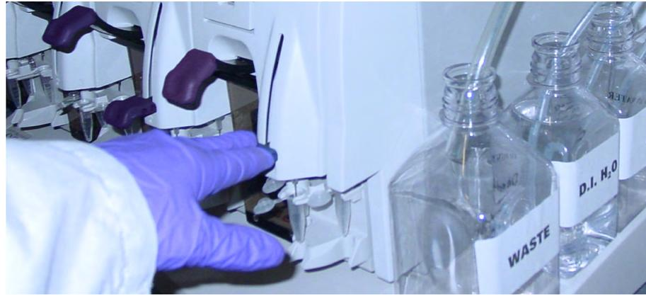
**Figure 4.15** The sample vials on the sample holder with the needle lever down — note the orientation of the vial caps.
