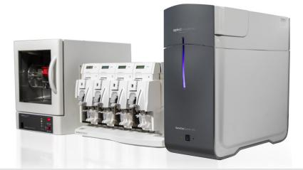
Do not attempt to monitor the thermal performance of the oven using temperature probes other than what is provided in the kit. The temperature profile is calibrated at the factory to facilitate proper operation.
