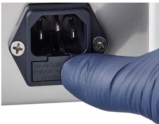
Figure 20 Returning the fuse holder
