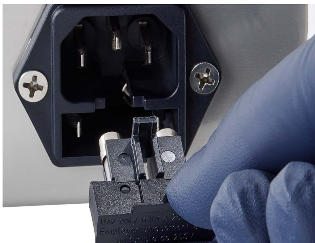
Figure 19 Removing the fuse holder
