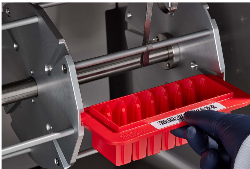
Figure 14 Slide the carrier into the rotisserie.
