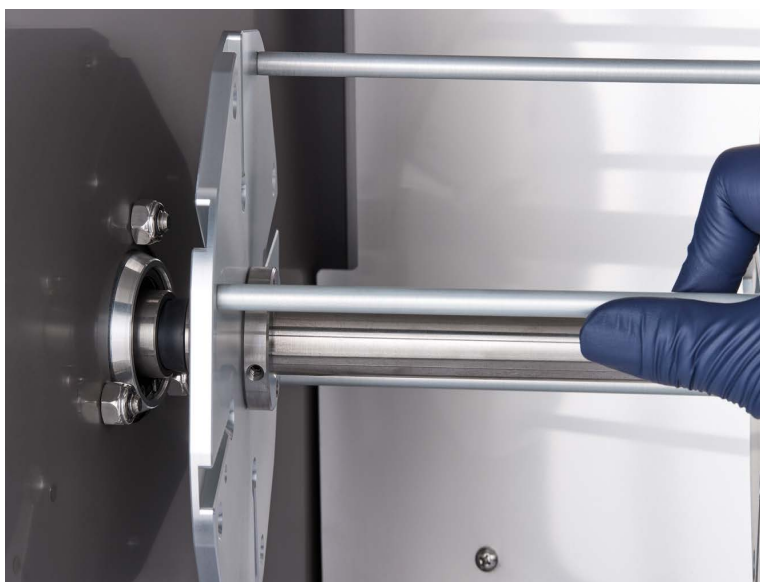
Figure 4 Installing the rotisserie into the left socket.
