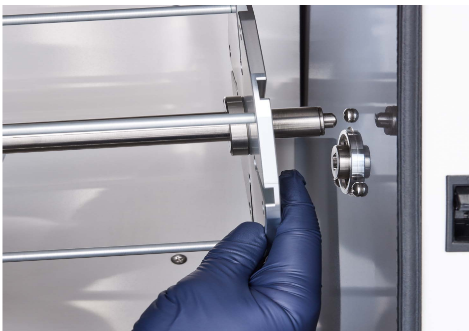
Figure 5 Installing the rotisserie on the right holder.
