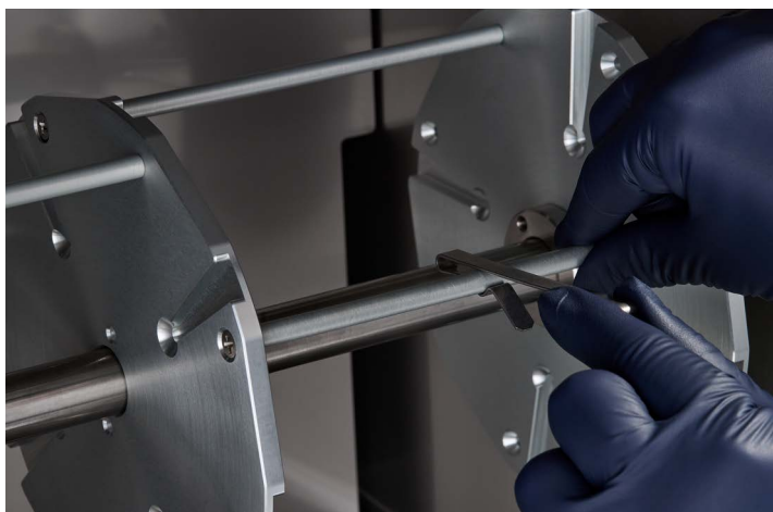
Figure 13 Installing the carrier retaining clips at the center of the crossbars.
