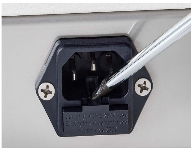
Figure 18 Use a screwdriver to remove the fuse holder located under the 3-pronged plug.
