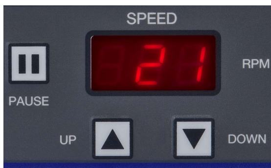
Figure 11 The rpm display and UP/DOWN keys.
