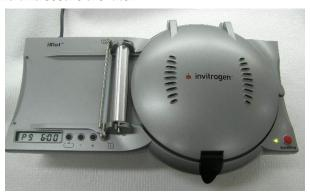
4. Press the Start/Stop Button to start the second (primary antibody) step. The two horizontal bars stop flashing.
