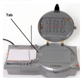
4. Clean the Metal Spacer 1 with a damp cloth or tissue and place the spacer on the membrane as shown below.
