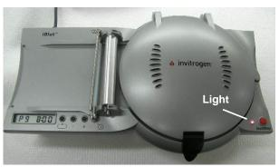
3. Select program P9. This program is a 3-step program for the iBlot® Western Detection protocol. The complete program runs for 8 minutes, and cannot be modified.
