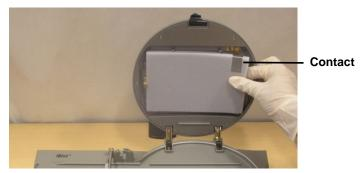
The sponge absorbs any excess liquid generated during blotting and exerts an even pressure on the stack surface.
