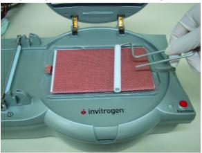
8. Position the Disposable Sponge so the metal contact is at the upper-right corner of the lid. Proceed to **Performing Blotting**.
