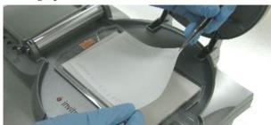
7. Remove any bubbles using the Blotting Roller.
