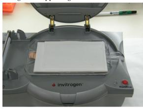
5. Remove any air bubbles using the Blotting Roller.
