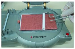
10. Place the iBlot<sup>®</sup> Disposable Sponge on the inner side of the lid (between the small protrusions on the lid that hold the sponge in its place) such that the metal contact is to the top right as shown below.
