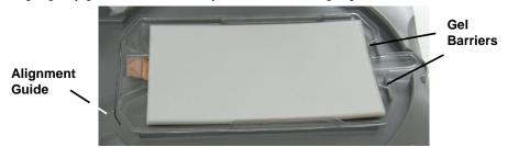
6. Use forceps to place the pre-wetted membrane on the Bottom Stack with the protein side facing up.
