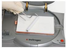
8. Remove the iBlot® Cathode Stack, Top (or Cathode Stack, Mini) from the package. Discard the red plastic tray.
