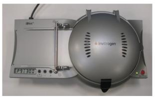
4. Press the Start/Stop Button to start the third (secondary antibody) step. The three horizontal bars stop flashing.
