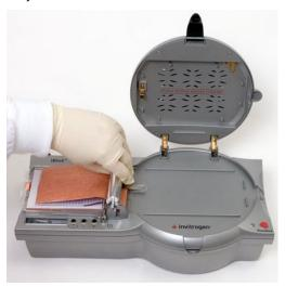
11. Hold the iBlot® E-PAGE™ Tab and plastic tab on the iBlot® Anode Stack, Bottom together and pull the assembly (anode stack, cathode stack, and gel) together through the De-bubbling Roller towards the blotting surface in one smooth, uninterrupted movement until the assembly reaches the Gel Barriers on the blotting surface (figure A). At the end of de-bubbling, all layers are aligned to the right as shown below (figure B).
