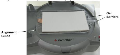
4. Place the gel on the transfer membrane (of the anode stack) with wells facing up and align with upper edge of anode stack.
