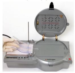
6. Clean the Metal Spacer 2 with a damp cloth or tissue and place the spacer over the gel as shown below.
