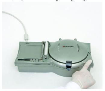
12. Current automatically shuts off at the end of each run. The end of transfer is indicated by beeping sounds, flashing red light, and digital display. Press and hold the Start/Stop Button. The light turns to a steady red and the beeping stops.
