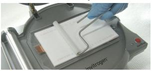
8. Use forceps to place the matrix soaked with Antibody Diluent Mix (Step 3) onto the membrane.
