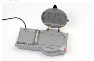
2. Remove the sealing of the iBlot<sup>®</sup> anode stack (Bottom). Keep the stack in the plastic tray.
