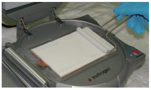
10. Remove the sealing from the iBlot® Western Detection Top Stack. **Keep the red plastic tray** for Step 16.
