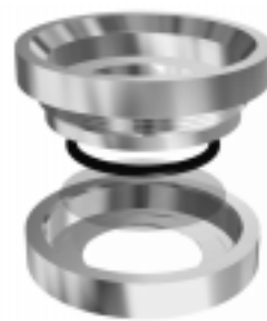
Figure 4. The Attofluor cell chamber (A-7816) is a durable and practical coverslip holder designed for viewing live cell specimens on upright or inverted microscopes. The cell chamber is constructed from surgical stainless steel, which allows accurate temperature control when used on a heated microscope stage, and is autoclavable, allowing cells to be grown directly in the chamber. The cell chamber mounts in a standard 35 mm-diameter stage holder, while the thin 0.5 mm base thickness allows clearance for the objective when focusing. The open, beveled design facilitates microinjection or electrophysiological procedures.
