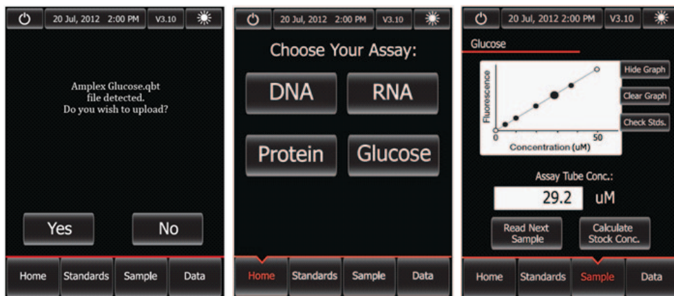
Figure 2 Upload of the MyQubit Amplex® Red Glucose assay. The Qubit® 2.0 Fluorometer will recognize the Amplex Glucose.qbt file and guide you through the upload process.
