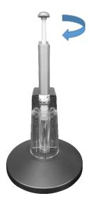
7. When the SUS Head is assembled, the appearance of the pipette should be adjusted so that the ① and ② are collinear.
