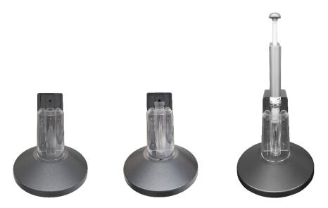
2. Rotate the Neon™ Pipette counterclockwise; then, hold the SUS Head by hand to disassemble it completely.
