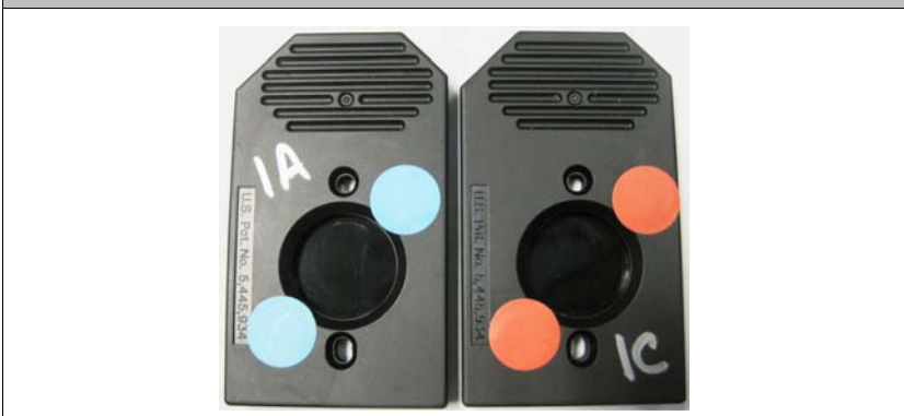
Figure 6.27 Covering the septa with Tough-Spots® that overlap the window
