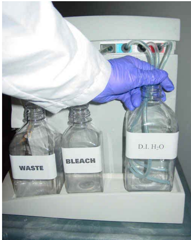
Figure 8.5 Immerse the Three Wash and Water Lines in the DI Water Bottle
