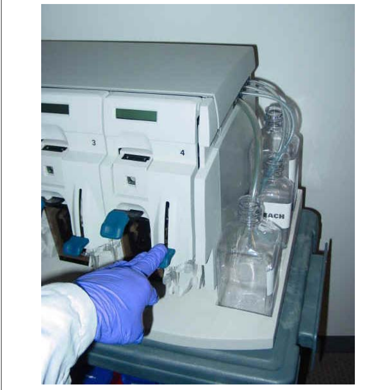
Figure 8.4 Press Down on the Needle Levers to Start the Bleach Protocol
