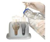
3. Pour sterile PBS into the Elution Vessel to the fill line (35 mL).
