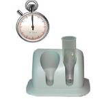
6. Leave the Elution Vessel in the rack for 1 min to allow the beads to be collected on the magnet.
