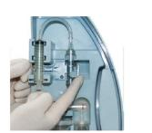
7. Slide the magnet assembly into locking position and check that it will release using the button on the side of the cartridge.
