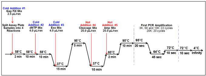
Figure 3.42 Meg 3-5-10K and Meg 20K Thermal Cycler Programs
