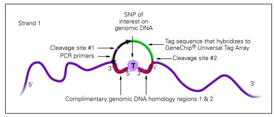
Figure 3.25 Assay Panel Probe Annealed to Genomic DNA Sample
