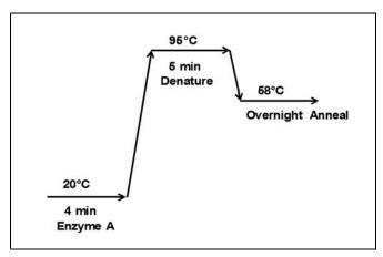
Figure 3.30 Meg Anneal Thermal Cycler Program
