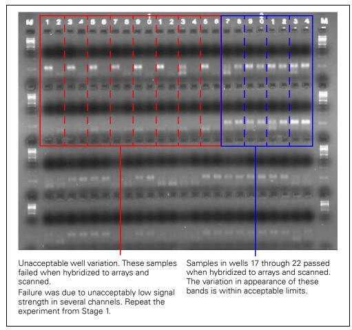
Figure 3.50 First Quality Control Gel with Mixed Results
