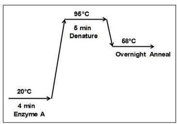
Figure B.1 Meg Anneal Thermal Cycler Program
