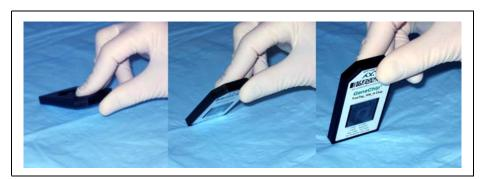
Figure 3.68 Swiping an Array to Dispel Air Bubbles
