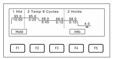
**Figure B.22P**Thermal Cycler Display for the Meg Hypcr 3-5k Program
