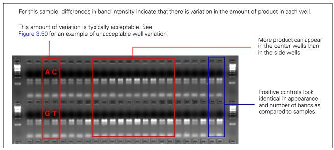
Figure 3.49 Good First Quality Control Gel for Assay Panel run on a 10K Universal Tag Array - Top Half Only
