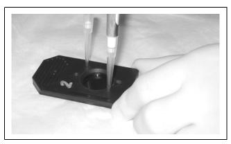
Figure 3.61 Loading Sample Onto an Array
