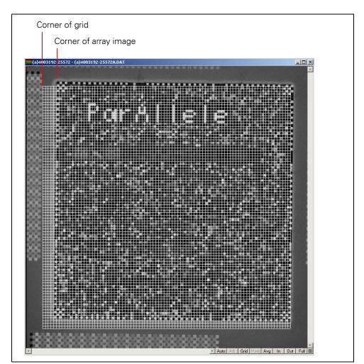
Figure 4.18 shows a .dat file that did not grid properly. You can see how the grid is not aligned with the edges of the array image.
