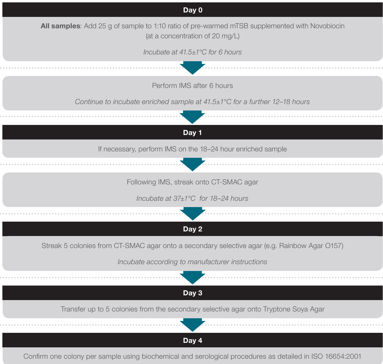
Figure 3. ISO 16654:2001 Reference method for the detection of E. coli O157:H7 from fresh spinach.
