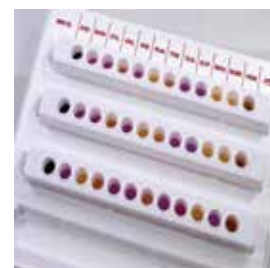
Oxid Microbact™ Listeria 12 L test strips in a holding tray
