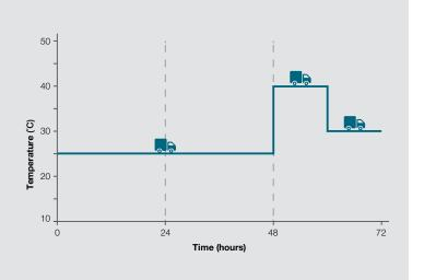
Transportation studies, designed to simulate real European transportation parameters, were conducted as part of ISO 15189 certification according to SOP BT-SOP-6958 (25°C for 48 hours, followed by 35-39°C for 8 hours, followed by 30°C for 16 hours) to prove stability of performance through product shelf-life following simulated transport times and temperatures.
