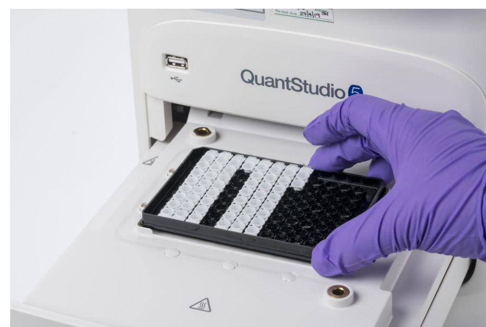
Figure 2. Thermo Scientific SureTect PCR Tubes being loaded in the QuantStudio 5 Food Safety PCR Instrument
