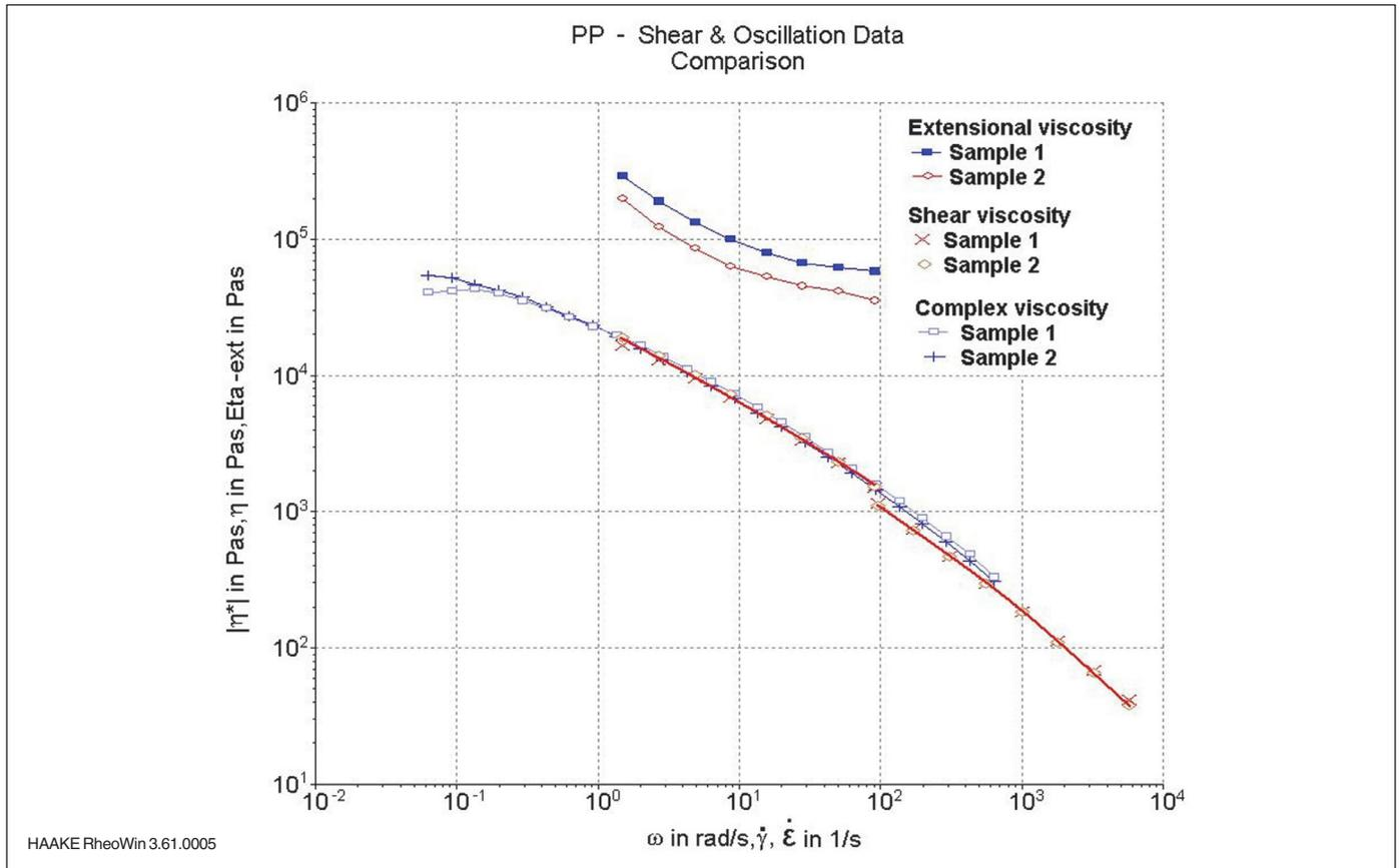
Figure 2: Viscosity data in shear, elongation and oscillation.
