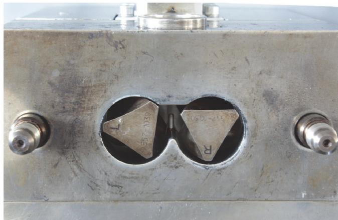
**Figure 1:** The chamber of the Rheomix Lab Mixer (600 OS version) with combined melt temperature and conductivity sensor.
