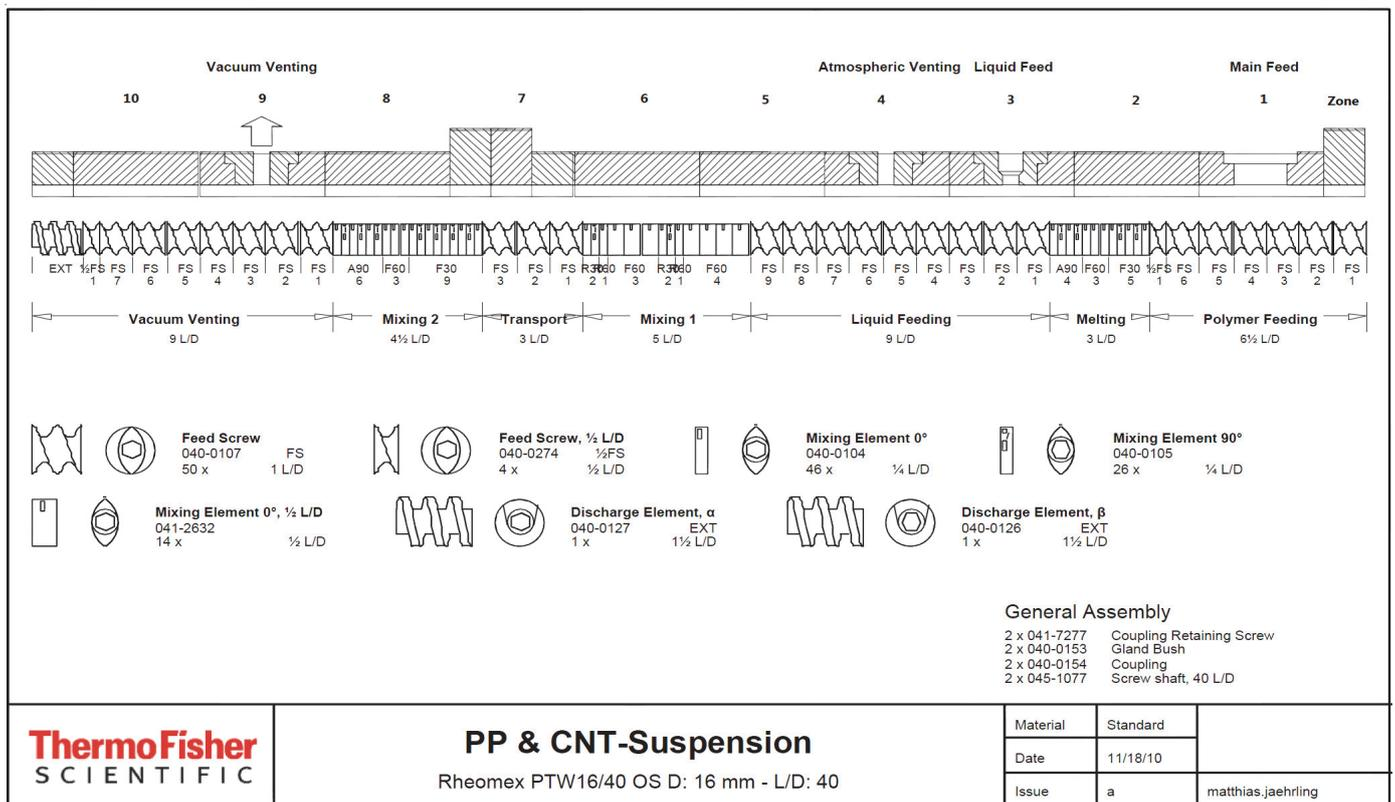
Fig. 1: Extruder- and screw configuration.
