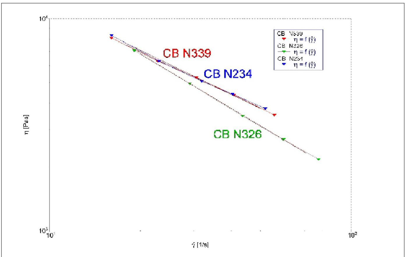
Fig. 9: The result of the viscosity measurements.
