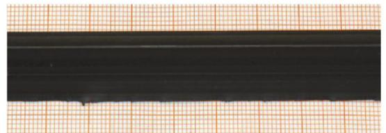
Fig. 3: Garvey profile examples of the 3 rubber formulations.
