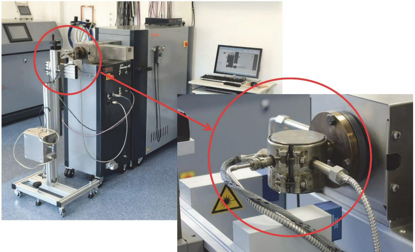
Fig. 4: HAAKE PolyLab OS setup with die-swell measurement.
