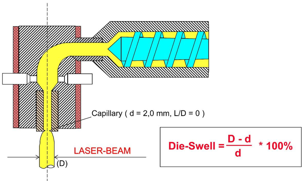
Fig. 5: Schematic and calculation of die-swell measurement.
