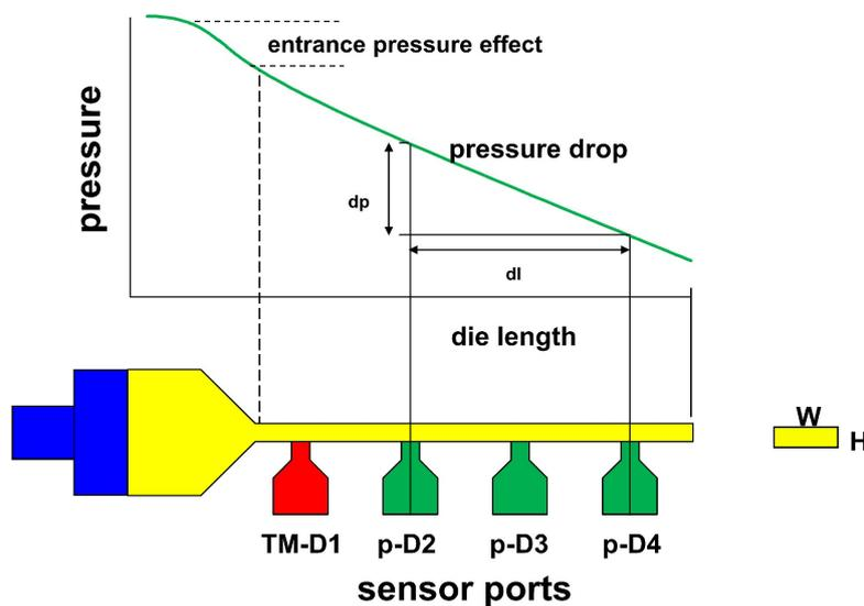
Fig. 7: Schematic of a horizontal slit capillary die.
