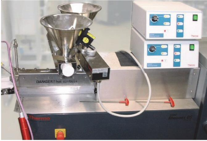
Fig. 2: Separate feed of wax and powder.
