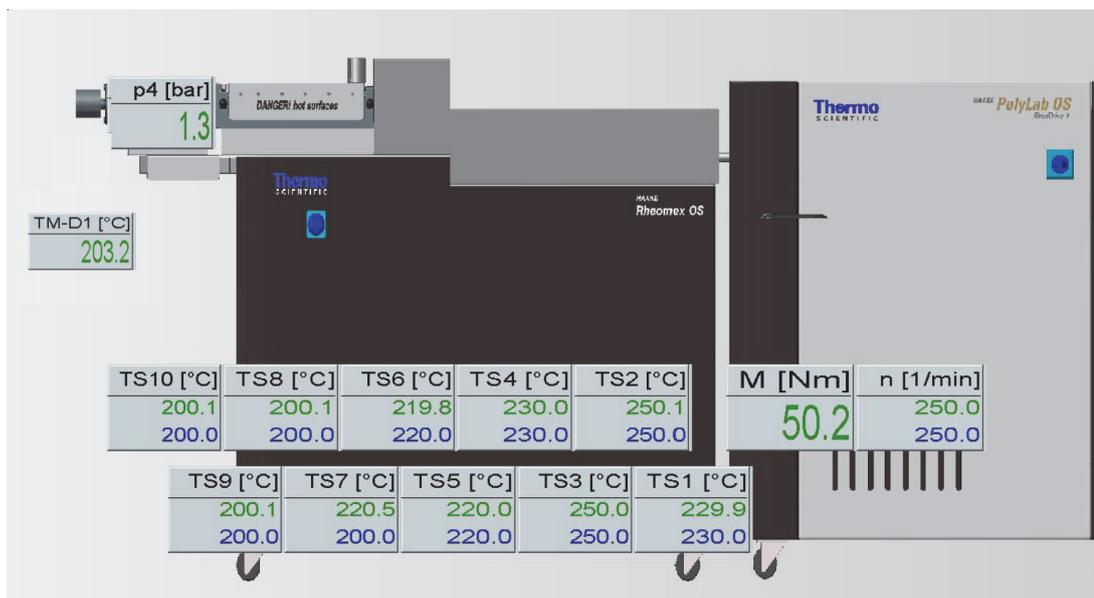
Fig. 2: Extrusion conditions.
