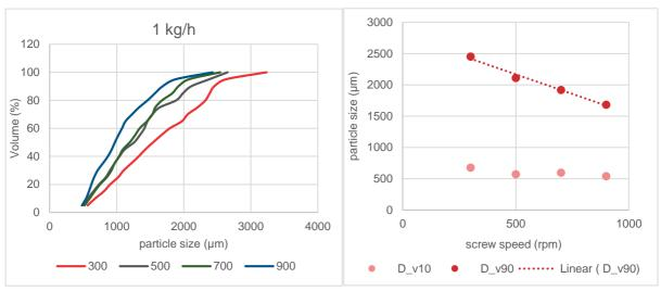
Figure 10 – Screw Speed Effect on PSD
