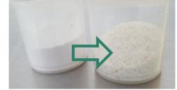
Figure 1 Material Before and After Granulation
