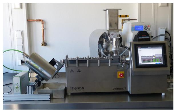
Figure 8 – Eyecon<sub>2</sub> Particle Analyser with Integration Device in-place on Pharma 11 Extruder in Granulation Mode (View 3)
