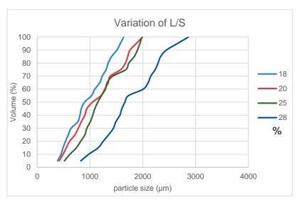
Figure 9 – L/S Ratio's Effect on PSD
