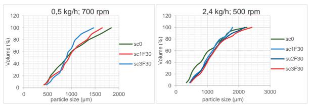
Figure 15 – Kneading Zone's Effect on PSD (low throughput rate)
