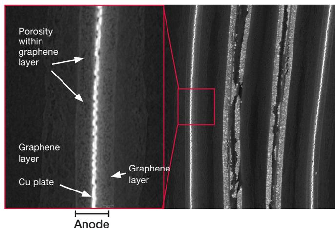
Figure 3. microCT-based 2D visualization of the anode internal structure.
