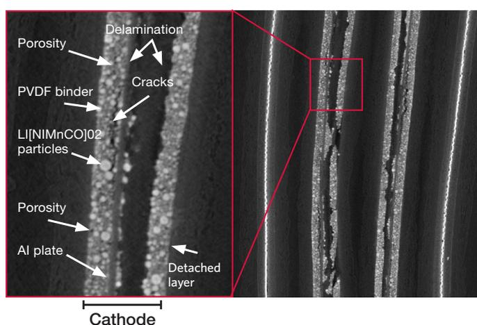
Figure 4. microCT-based 2D visualization of the cathode internal structure.
