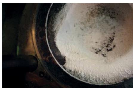
Figure 1. Piston top coated with SiO<sub>2</sub>.
