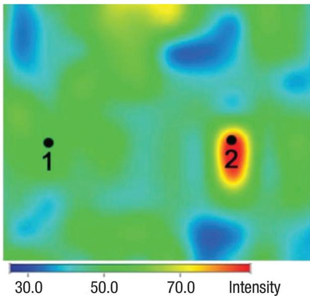
**Figure 4.** A Raman map showing the distribution of the two different spinel phases in a sample. The red-yellow locations (such as location 2) indicate areas of the  $\text{P}4_3\text{3}2$  phase whereas the blue-green areas (such as location 1) represent areas of the  $\text{Fd}3\text{m}$  phase. Mapping data collected using a DXR Raman Microscope with a motorized stage and Atlaps software. Adapted with Permission from Zhang X, Cheng F, Zhang K et al. (2012) *RSC Advances* 2: 5669–5675.
