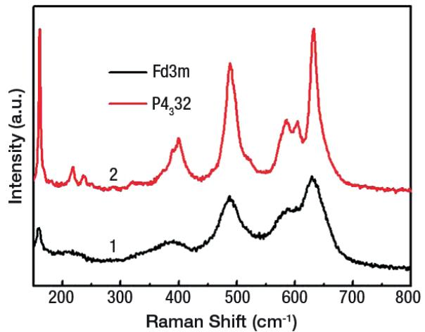
Figure 1. Raman spectra of the two phases of  $\text{LiNi}_{0.5}\text{Mn}_{1.5}\text{O}_4$ . Spectra were collected using a DXR Raman Microscope and a 532 nm laser. Adapted with permission from Zhang X, Cheng F, Zhang K et al. (2012) RSC Advances 2: 5669–5675.
