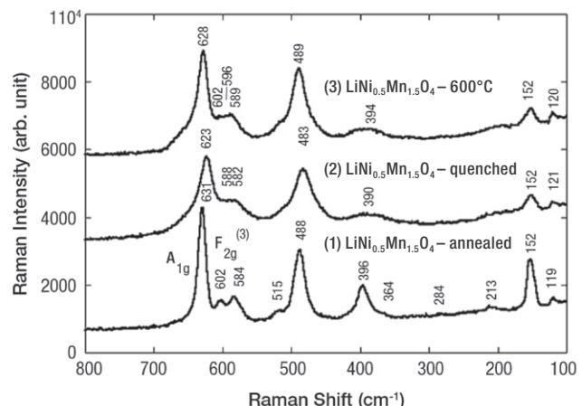
Figure 2. Raman spectra of  $\text{LiNi}_{0.5}\text{Mn}_{1.5}\text{O}_4$  synthesized under various conditions. (1) Annealed at high temperature, (2) quenched, and (3) calcined at lower temperature. Spectra were collected using a Thermo Scientific™ Nicolet™ Almega™ XR dispersive Raman spectrometer equipped with a 633 nm laser. Adapted with permission from Oh SH, Chung KY, Jeon SH et al. (2009) Alloys Compd 409: 244–250.
