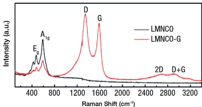
Figure 6. The Raman spectra of  $\text{Li}(\text{Li}_{0.2}\text{Mn}_{0.54}\text{Co}_{0.13}\text{Mn}_{0.13})\text{O}_2$  (LMNCO) and the graphene enwrapped hybrid material (LMNCO-G). Spectra were collected using a DXR Raman Microscope and a 532 nm laser. Adapted with permission from Jiang K-C, Wu X-L, Yin Y-X et al. (2012) *ACS Appl Mater Interfaces* 4(9): 4858–4863.
