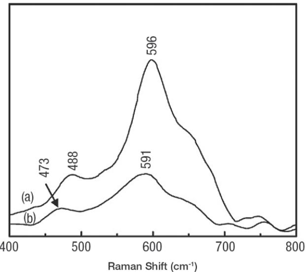
**Figure 5.** The Raman spectra of (a)  $\text{Li}_{1.15}[\text{Mn}_{0.45}\text{Co}_{0.40}\text{Ni}_{0.15}]\text{O}_2$  and (b)  $\text{Li}[\text{Mn}_{0.45}\text{Co}_{0.40}\text{Ni}_{0.15}]\text{O}_2$ . Peak shift and intensity change with change in lithium content. Spectra collected using a Nicolet Almega XR dispersive Raman spectrometer configured with a 532 nm laser. Adapted with permission from Wang T, Liu Z-H, Fan L et al. (2008) *Powder Technol* 187: 124–129.
