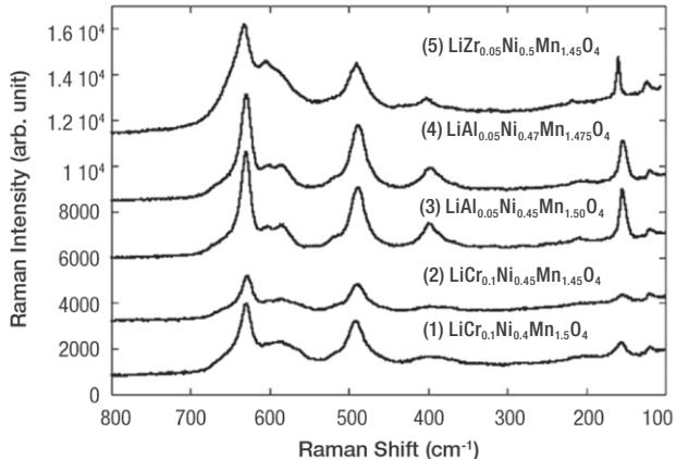
**Figure 3.** Raman spectra of Zr, Al, and Cr doped  $\text{LiNi}_{0.5}\text{Mn}_{1.5}\text{O}_4$ . (1) and (2) Cr doped ( $\text{Fd}3\text{m}$  structure); (3) and (4) Al doped ( $\text{P}4_3\text{3}2$  structure); (5) Zr doped ( $\text{P}4_3\text{3}2$  structure). Spectra were collected using a Nicolet Almega XR dispersive Raman spectrometer configured with a 633 nm laser. Adapted with permission from Oh SH, Chung KY, Jeon SH et al. (2009) *Alloys Compd* 409: 244–250.
