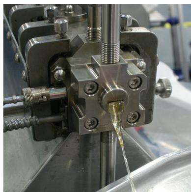
Figure 3: Extruder with transmission probes attached
