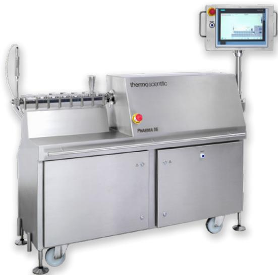
Figure 1. Pharma 16 Twin-Screw Extruder.
