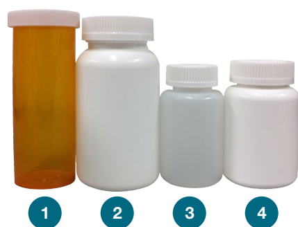
Figure 1. Pharmaceutical bottles selected for testing: bottle 1 – amber translucent container, bottle 2 – large white opaque container, bottle 3 – natural translucent container, bottle 4 – small white opaque container.
