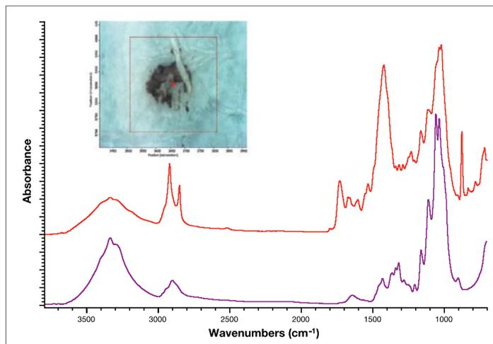
**Figure 4: Using micro-ATR to investigate possible contaminants and particles in an unprinted area of 20 Euro note. Upper trace is the spectrum of an embedded particle in the paper matrix; lower trace is the paper region just adjacent to the particle.**
