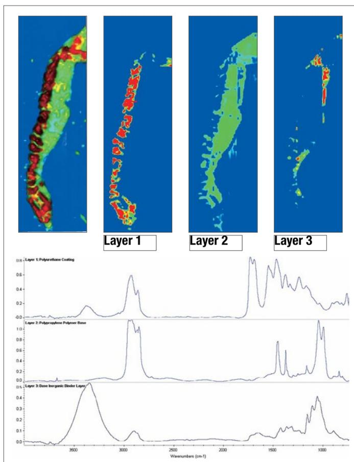
**Figure 7: (Upper) Chemical image of a car bumper paint chip layers. (Lower) Spectra of identified layers: Layer 1: protective coating. Layer 2: base coat and polypropylene polymer, Layer 3: binder layer.**
