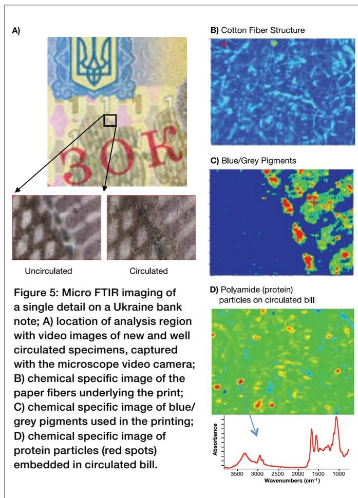
**Figure 5: Micro FTIR imaging of a single detail on a Ukraine bank note; A) location of analysis region with video images of new and well circulated specimens, captured with the microscope video camera; B) chemical specific image of the paper fibers underlying the print; C) chemical specific image of blue/grey pigments used in the printing; D) chemical specific image of protein particles (red spots) embedded in circulated bill.**
