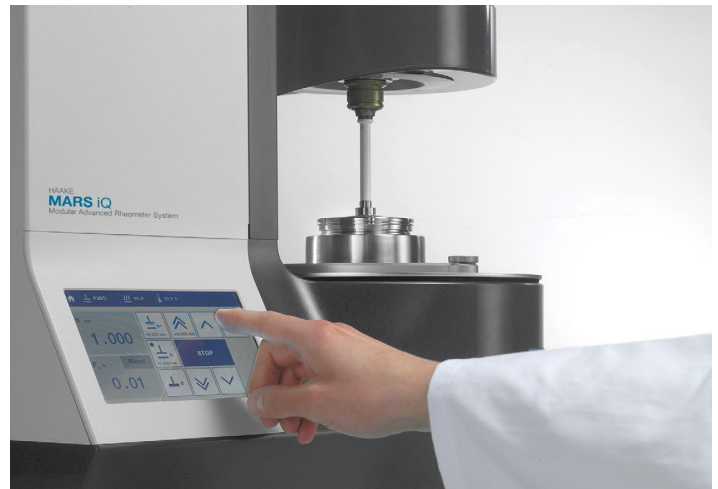
Figure 3: Execution of a standardized measuring and evaluation routine directly at the rheometer
