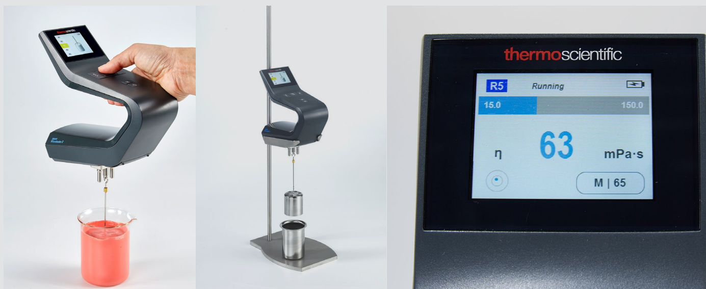
Figure 1: HAAKE Viscotester 3 Viscometer as hand-held device (left), with laboratory stand (middle) and detailed view of the display with measured value and comparison with reference value (right)
