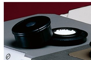
Figure 2: Antaris II analyzer with the closed sample cup and spinner
