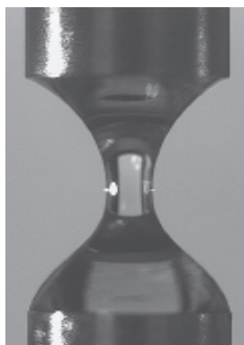
Fig. 2: Sequence of a CaBER measurement.
