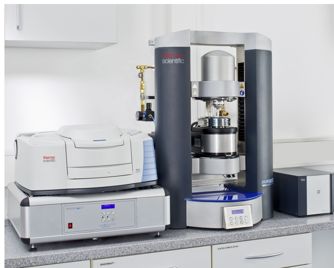
Fig. 1: The HAAKE MARS rheometer with Rheonaut module and Nicolet iS 10 FT-IR spectrometer.
