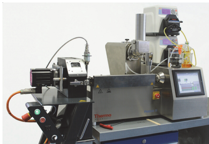
Fig. 1: Thermo Scientific Process 11 "Hygienic" with face-cut pelletizer.
