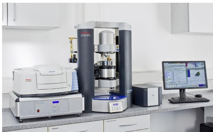
**Figure 1: Setup with the HAAKE MARS Rheometer, Rheonaut module\* and FTIR spectrometer.**
