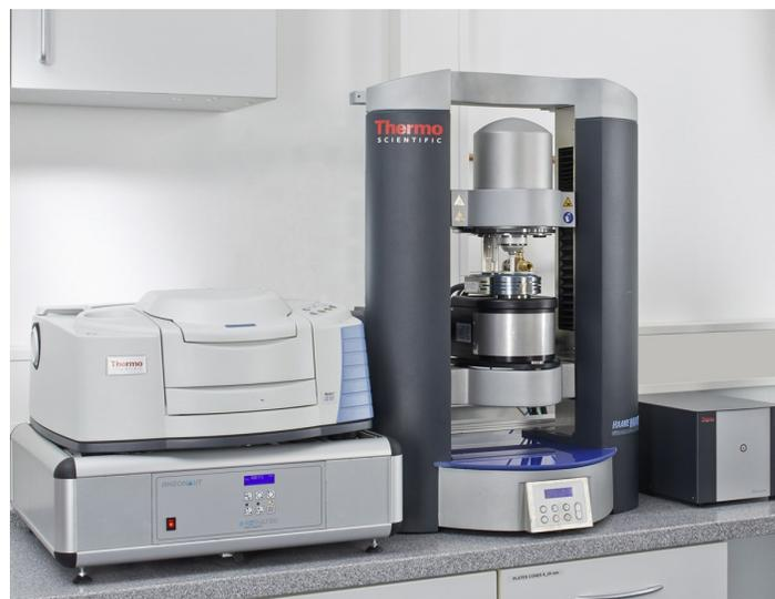
Figure 1: Setup with HAAKE MARS Rheometer, Rheonaut module and FT-IR spectrometer.
