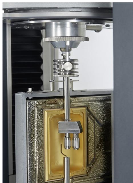
Figure 1: SER3 tool with HAAKE MARS Rheometer and CTC.
