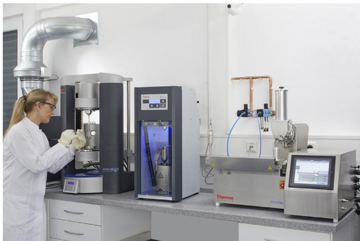
**Figure 2: Polymer workflow (from right to left) Mini compounder, injection molding system to produce test specimens and HAAKE MARS 60 Rheometer with controlled test chamber for polymer tests in a temperature range between -150 °C up to 600 °C.**
