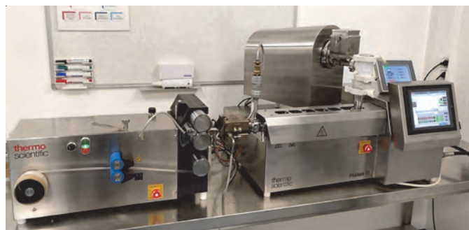
Figure 1: Benchtop system including a Pharma 11 Twin-Screw Extruder for production of ODFs.
