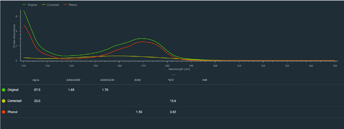
Figure 2. RNA spectra with phenol contamination, identified by Acclaro Technology. The NanoDrop One/One c software reports the corrected RNA concentration and spectrum in yellow.
