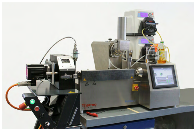
Figure 1: The Thermo Scientific Process 11 "Hygienic" Parallel Twin-Screw Extruder
