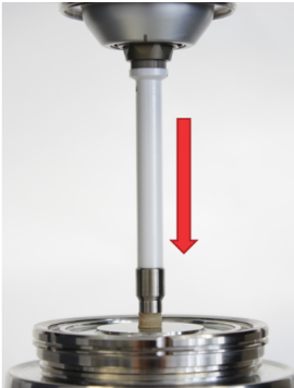
Figure 3: Measurement setup for compression tests using a HAAKE MARS 60 Rheometer and plate-plate geometry P8.
