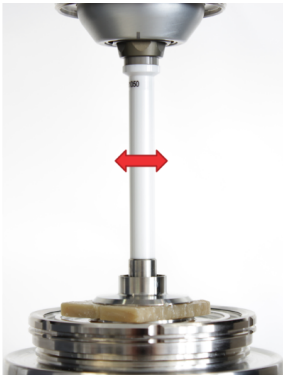
Figure 4: Measurement setup for amplitude and frequency (bulk) using a HAAKE MARS 60 Rheometer and plate-plate geometry P35.
