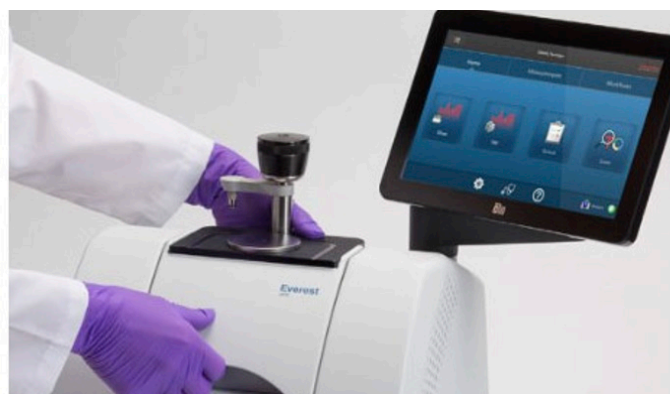
Figure 5: Nicolet Summit PRO FTIR Spectrometer with Everest ATR accessory and on-board touchscreen monitor
