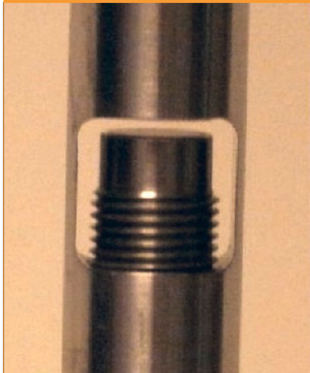
FIGURE 2: Transflectance probe used in the analysis, showing detail of adjustable pathlength.
