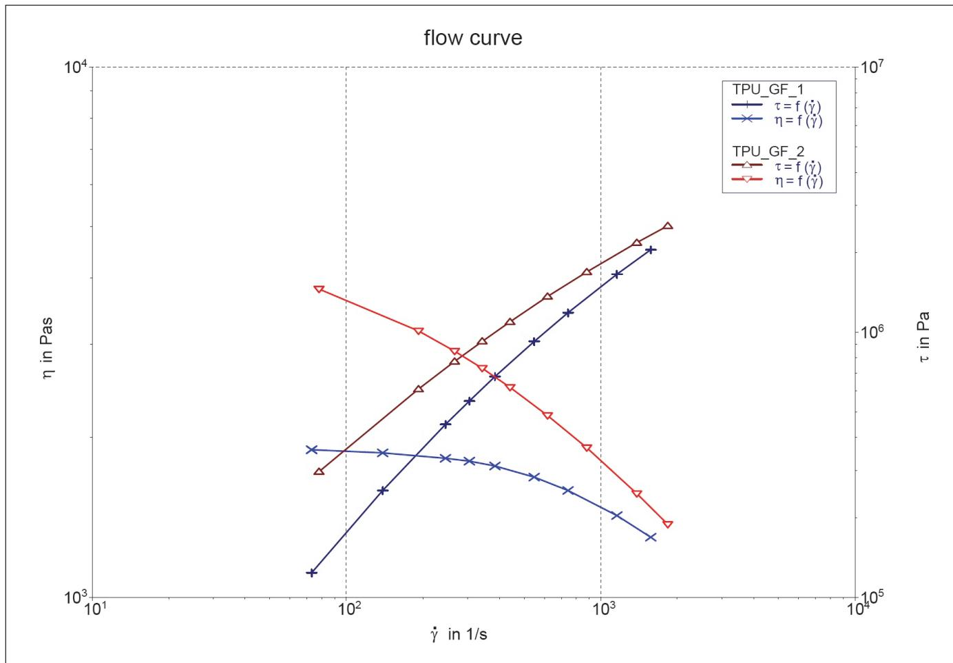
Figure 1: Superimposed test results for two TPU samples.
