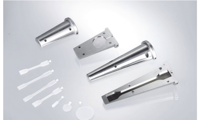
Fig. 4: Tensile bar in HAAKE MiniJet Pro mould.
