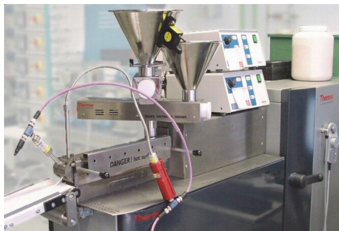
Fig. 1: Instrument setup, RheoDrive 16, PTW16/25, split feed with two metering feeders, die plate and conveyor belt.
