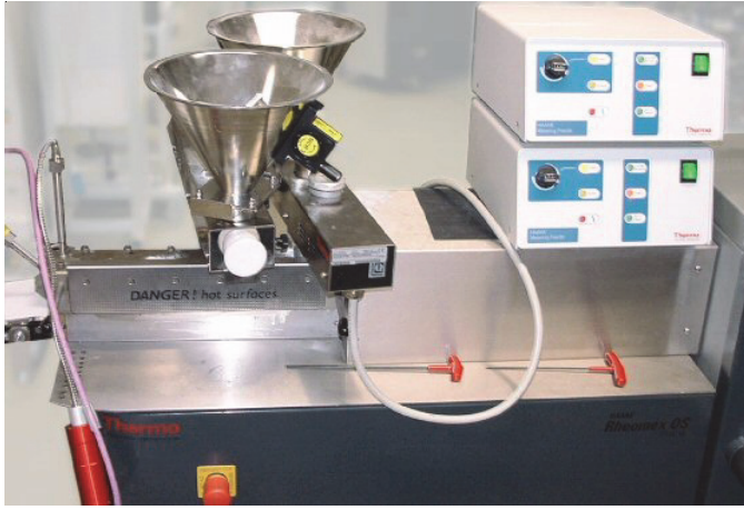
Fig. 2: Separate feed of wax and powder.
