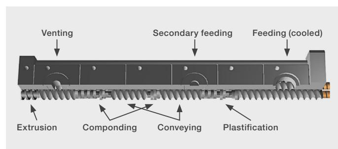
Figure 2: Schematic of a twin-screw extrusion.
