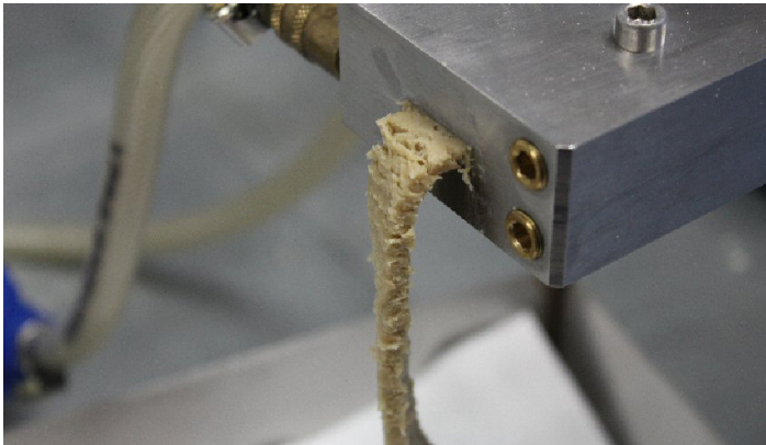
Figure 2: Special die for the extrusion of plant-based proteins samples.
