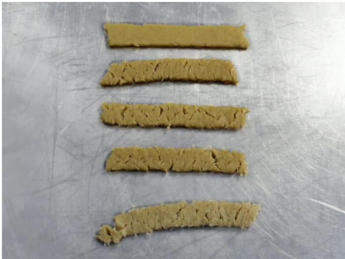
Figure 3: Wheat gluten samples with different textures. From top to bottom: The samples develop the fibrous characteristic of meat by optimizing the extrusion conditions.
