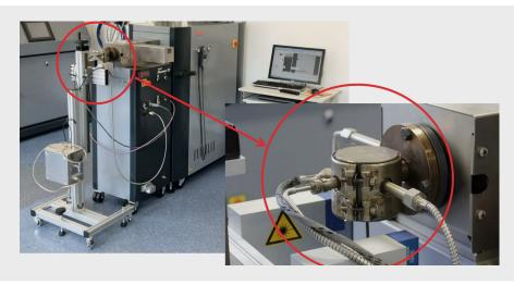
Figure 4: HAAKE PolyLab OS setup with die-swell measurement.
