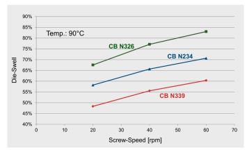
Figure 6: Die-swelling phenomena for three rubber formulations.
