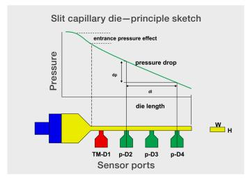
Figure 7: Schematic of a horizontal slit capillary die.
