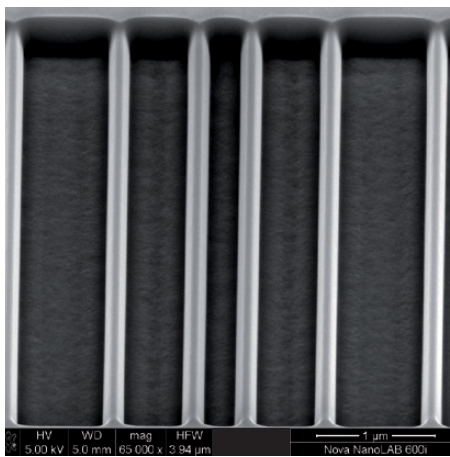
Figure 16. The Thermo Scientific parallel multi-pass milling strategy delivers a smooth bottom and clean sidewalls for all pattern elements.
