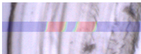
Video Image of the cross-section; FTIR image superimposed showing Nylon 6 layers
