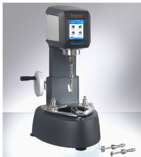
Figure 1: The HAAKE Viscotester iQ Rheometer with universal container holder and vane rotors for relative measurements.
