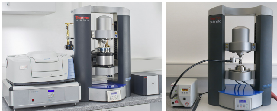
Figure 1: left: HAAKE MARS Rheometer with Rheonaut module and FTIR spectrometer; right: HAAKE MARS rheometer configuration for UV-curing measurements incl. temperature control.
